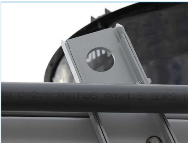
Use shackles in lifting ears to lift the unit
