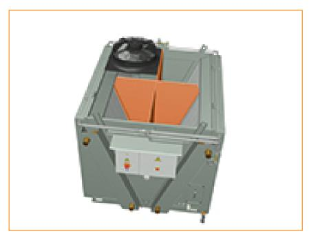
Equipping a unit with partition panels provides an **individual air intake duct for each and every fan** on the adiabatic cooler. This guarantees a higher capacity in case of fan failure by avoiding unintended air flows through an idle fan which bypasses the coil.
