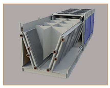
Equipping a unit with partition panels provides an **individual air intake duct for each and every fan** on the adiabatic cooler. This guarantees a higher capacity in case of fan failure by avoiding unintended air flows through an idle fan which bypasses the coil.
