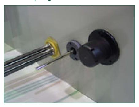
Our factory-installed heaters keep the water temperature at 4°C and act as a simple and economical **anti-freeze measure for the basin water**. The heater package includes the **heaters**, a **thermostat** and a **low level cut out switch** to protect the heaters if the water level declines excessively. Standard electric heaters can handle ambient temperatures down to -18°C.
