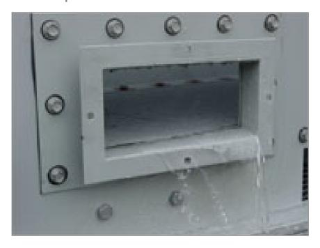
A factory-installed clean out port
