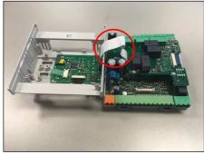
Step 3: Remove the circuit board. First remove 4 screws holding the circuit board and slide the circuit board horizontally to the back to release the connecting strip which sits in a slot in the circuit board. Carefully flip the circuit board to the right side. It is also connected with wires to the main circuit board.
