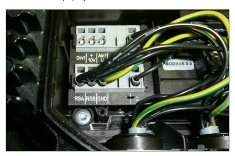
Measure the resistance between terminals NC and C. Is this an open contact or a closed contact?
